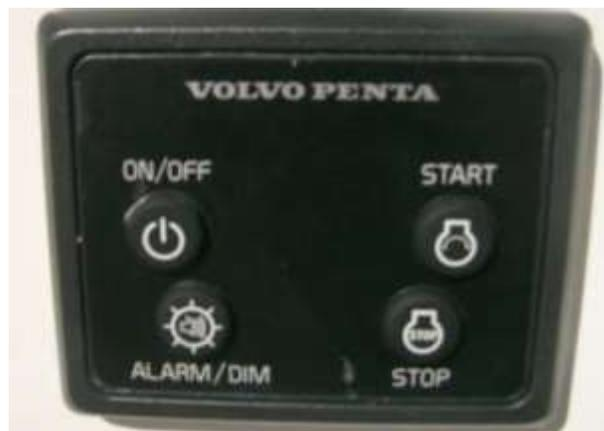
Maintain engine RPMS below 1800. **MAXIMUM ENGINE REVS 2200 RPM**
