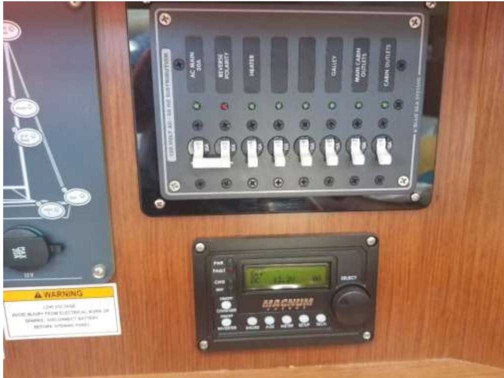
To avoid additional drain on your batteries while operating electrical appliances, the engine should be turned on and revved up to 1400 rpm IN NEUTRAL. Make sure that the inverter is turned off at all times when not in use.
