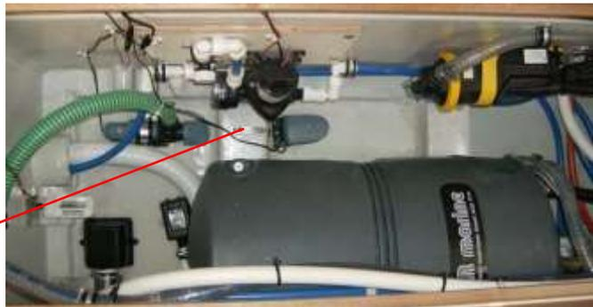
Manual bilge pump located aft of starboard helm
